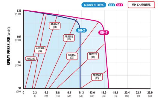
FLOW RATE kg/min (lbs/min)
